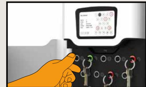
All keys and keysets are individually locked by the Traka21 unit. Green LEDs indicate those keys to which this user has access. The user cannot remove keys highlighted by the Red LEDs which continue to remain locked in place.
