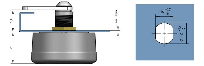
2. Fastening in wooden doors by means of cup drilling and optional anti-rotation bolt (Specify when ordering)
