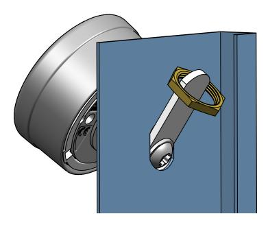
2. Assembly sequence for separately delivered cams
