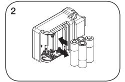
Remove the batteries from the housing. Replace with four premium alkaline AA batteries. Dispose or recycle used batteries according to local regulations.
